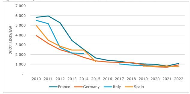
Figure 10: Utility-scale solar PV total installed cost trends in selected countries
