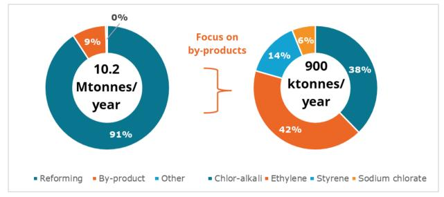
Figure 60: Hydrogen production capacity in the EU by process (2022)
